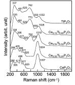
**Figure 2.** Raman spectra of the  $Ce_{1-x}Ti_xP_2O_7$  powders.
