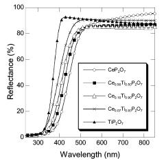
**Figure 1.** Optical reflectance spectra of the  $Ce_{1-x}Ti_xP_2O_7$  sunscreens having various Ce/Ti ratios.
